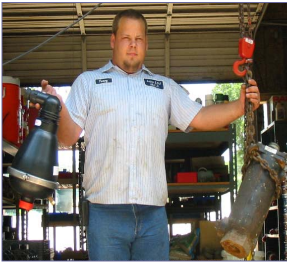
Conventional Valve beside ARI D-025 Weight Comparison
